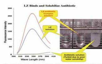
Fluorescence spectrum shows increase of intensity and shift to higher wavelength of LZ with 1.2
